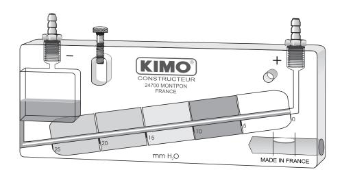
The CP 25 inclined liquid column manometer, developed and manufactured by KIMO measures slight variations in pressure, depression or differential pressure of air or gas. It is specially designed for checking clogging of filters in painting booths.
